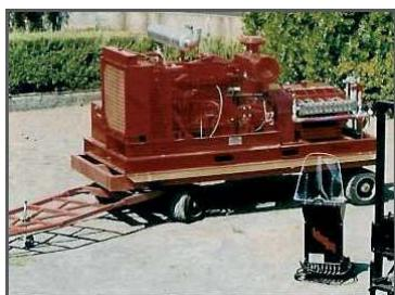
The base for heat exchangers cleaning is formed by a powerful high pressure Idrojet pump unit.
