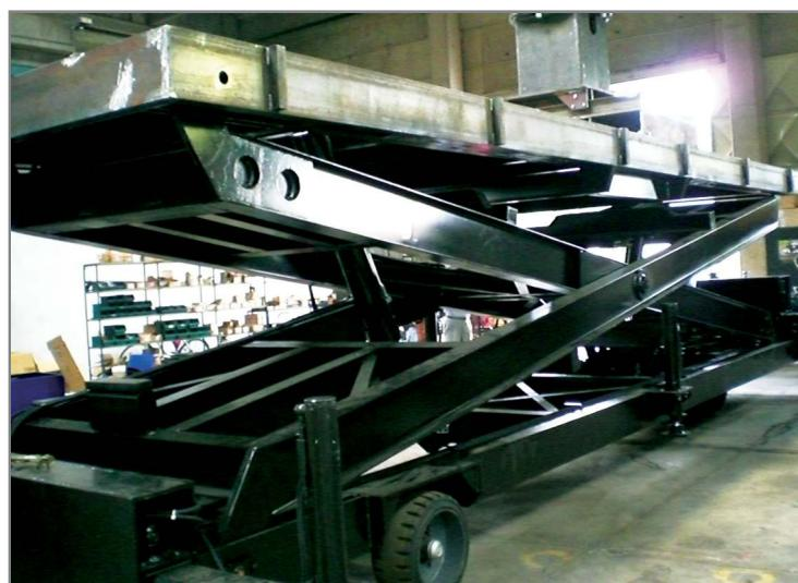
Model super-gas 1 for a max weight capacity of 10 ton at a maximum height of 7 mt.
