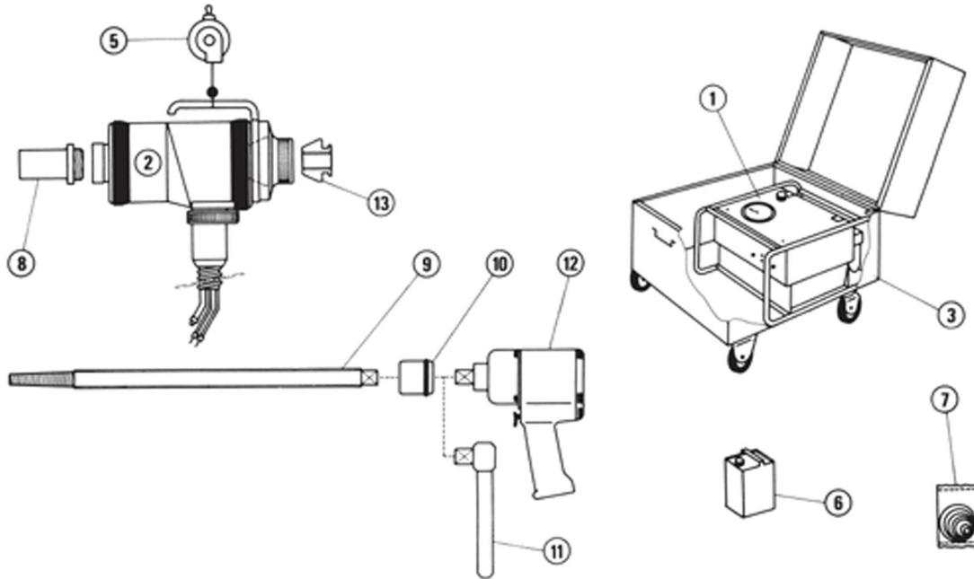
1 - HW 8000 air powerd hydraulic pump; 2 - HTP 500 gun(hydraulic clamping); 3 - Wheel mounted storage case ; 4 - Balancer; 5 - Special oil; 6 - Set of spare O-rings; 7 - HTP 300 collar (according O.D. tube); 8 - HTP 400 mandrel (according I.D. tube) ; 9 - Socket; 10 - Ratchet wrench (1" sqature drive); 11 - Impact wrench (1" square drive); 12 - Set of jaws (according to madrel diameter); 13 - Spare parts for 2 years service.
