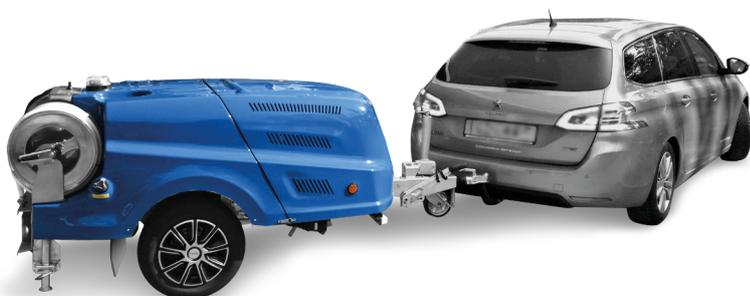
Version with "PLUS", multifunction radio control and hydraulic hose reel
