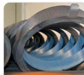
Freehanded rubber coating on nearly every surface
