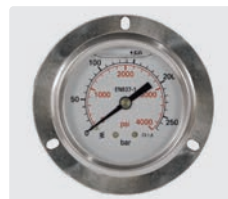
Ø 63 mm. 1/4" M. With mounting ring. Housing stainless steel. Inlet at the back
