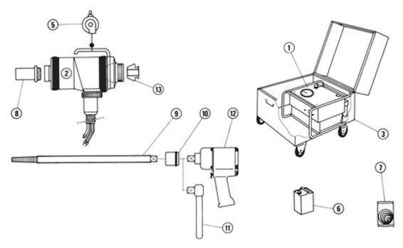
1 - HW 8000 air powerd hydraulic pump; 2 - HTP 500 gun(hydraulic clamping); 3 - Wheel mounted storage case; 4 - Balancer; 5 - Special oil; 6 - Set of spare O-rings; 7 - HTP 300 collar (according O.D. tube); 8 - HTP 400 mandrel (according I.D. tube); 9 - Socket; 10 - Ratchet wrench (1" square drive); 11 - Impact wrench (1" square drive); 12 - Set of jaws (according to madrel diameter); 13 - Spare parts for 2 years service.
