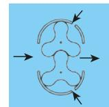
AIR INJECTION COOLING FOR ROTARY LOBE PUMPS
