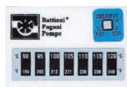
This temperature indicator provides two temperature readouts: The reversible scale at the bottom changes colour (from black to blue) at a specific temperature (90 °C to 120 °C). The scale is provided to help the user prevent the pump from overheating.
