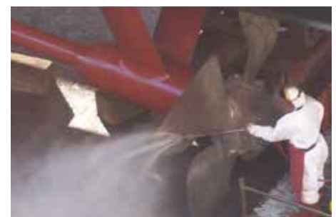
Removal of scale deposits and/or marine fouling
